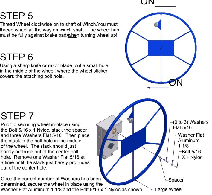
NOTE: You should be able to slide a piece of paper in the gap between sticker in the center of the wheel and the washer. The wheel should turn 1/8 to 1/4 turn prior to engaging the Washer Flat Aluminum 1 1/8.
