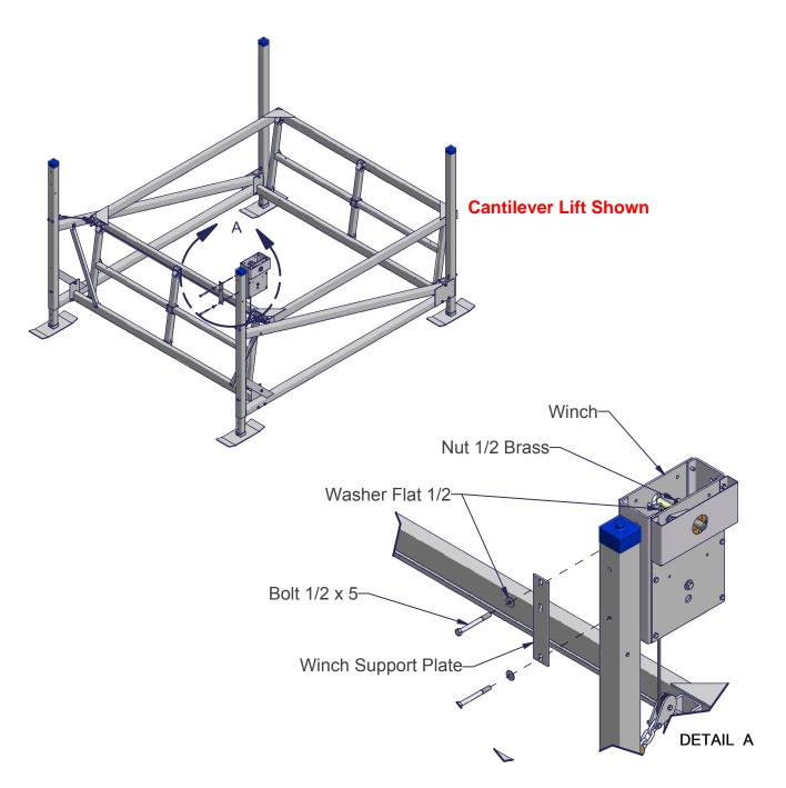
Slide end of cable into slotted opening on winch hub. Using a 3/16" Allen Wrench, tighten winch hub set screw to secure cable to winch hub.
